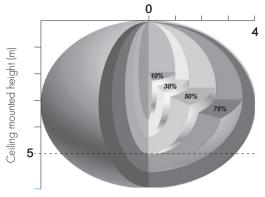
Ceiling mounted detection pattern (m)
