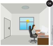
The sensor switches off the light The sensor switches off the light whenever natural light exceeds after the hold-time when there is pre-set daylight threshold, even no motion detected. with presence.
